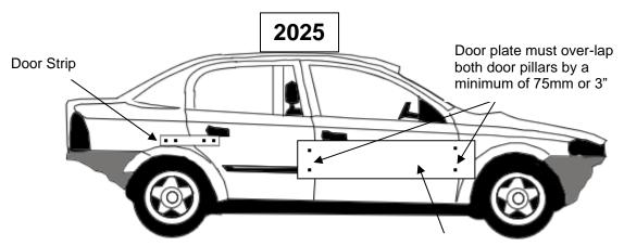
The Door plate must be fixed by either four 16mm or 19mm bolts or studs, through both the door pillars. No slotted holes allowed
